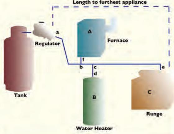
The diagram illustrates a gas distribution system. A gas tank feeds into a regulator. From the regulator, a main line (a-b) runs to a furnace (A). A branch (b-c) goes to a water heater (B), and another branch (c-d) goes to a range (C). The distance from the regulator to the range (e) is labeled as the 'Length to furthest appliance'. Points a, b, c, d, and e are marked along the piping.
