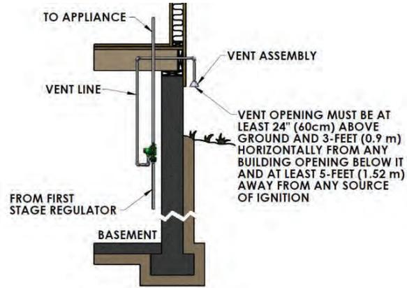
Figure 4: Basement Installation
