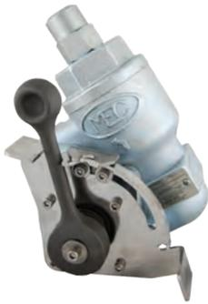
**Normal Bypass Mode:** functions just like our standard ME840 Series bypass valve during domestic tank deliveries by pushing maximum pump output to the hose end delivery nozzle while protecting the pump if the nozzle is closed during delivery.
