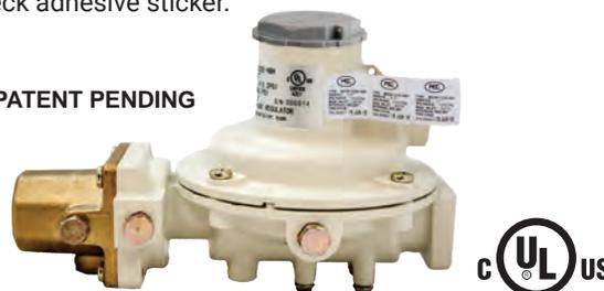
**MEGR-1232E Compact Series:** Offers a compact integral two-stage 2 PSI regulator design perfect for lower BTU applications and confined spaces. They feature an adjustment range from 1-2.2 PSI (factory set @ 2 PSI). Stainless steel integral components, fluorocarbon (FKM) seat discs, molded lip fabric reinforced diaphragms, and large precision machined aluminum orifices providing superior downstream regulation and maximum corrosion resistance against weather or contaminated gas.
