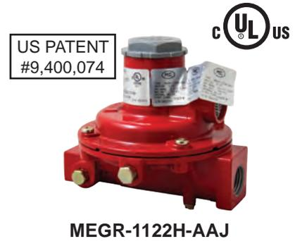
**MEGR-1122H Series:** Offers a compact first stage regulator design perfect for tight applications such as underground tank domes. They feature an adjustment range from 9-12 PSIG (factory set @ 10 PSIG), stainless steel internal components, fluorocarbon (FKM) seat discs, molded lip fabric reinforced diaphragms and large aluminum precision machined orifice to minimize freeze ups while providing superior downstream regulation and maximum corrosion resistance against weather or contaminated gas.
