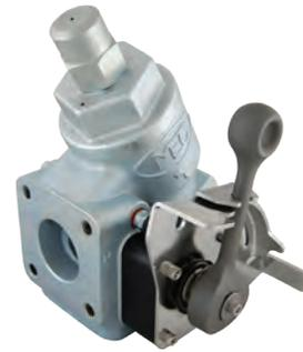
**Small Cylinder/Forklift Fill Mode:** a built in, fully adjustable proportional flow control valve allows a portion of flow from the pump to be diverted back to the tank in order to reduce flow rates at the hose end delivery nozzle to safely and accurately fill small cylinders.
