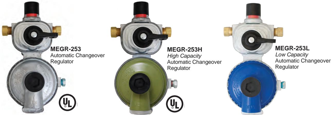
The **MEGR-253 Series** Automatic Changeover regulators automatically redirect LP gas vapor flow from an empty service cylinder to a reserve cylinder, without interruption of service. It features an easy to read green indicator which changes to red when the service cylinder needs to be refilled.
