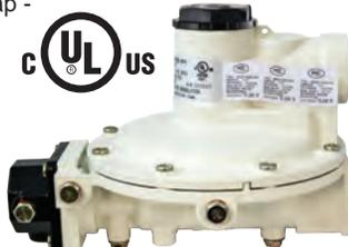
**MEGR-1632E Full Size Series:** Offers all of the same features as the compact MEGR-1232E series in a full size high capacity version. The full size MEGR-1632E diaphragm provides superior downstream regulation, has heavy duty wrench flats and a large 3/4" FNPT tapped drip lip vent to help prevent relief vent blockage.
