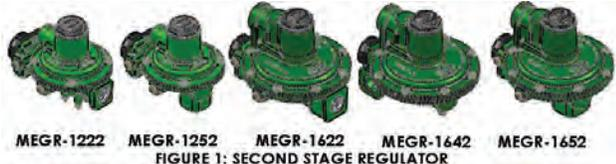
The second stage regulator is designed to reduce the outlet pressure from a first-stage regulator (usually 10 psig (0,69 bar)) to an outlet pressure of 11 -inches water column (27 millibars).
