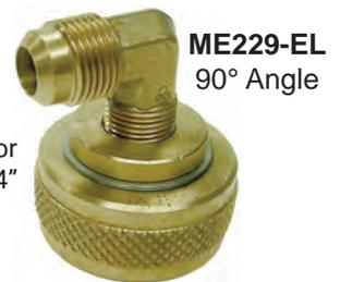
Enables the installation of a 1/4" MNPT hydrostatic relief valve in a safe, protected area. This two piece carburetion hose fitting fits all stainless steel braided LP-Gas hose with a 5/16" ID. The tank valve side has a 3/8" female flare swivel and zinc plated for maximum corrosion resistance.
