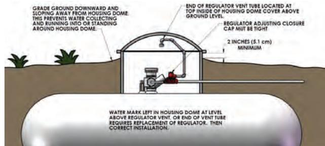
Figure 5: Underground Installation
