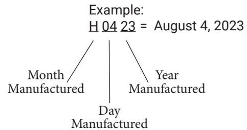
NOTE: Internal relief valves feature a different date code system.
